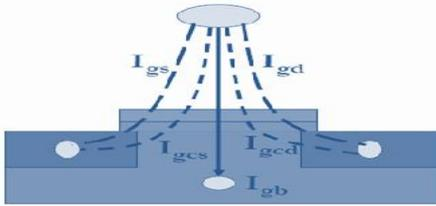
Fig.10: Static Power loss in CMOS Tunneling
