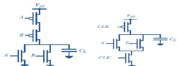
Figure 17.(a) : Static NOR Fig. 17(b) :Dynamic NOR
