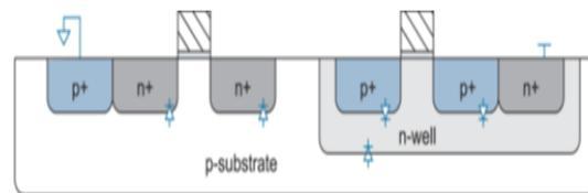
Fig.9: Junction Leakage due to Reverse Biasing
