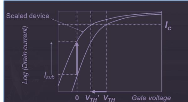
Fig.7 : Increased Sub threshold Leakage
