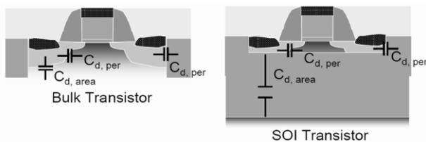
Fig.14: Capacitance Reduction
