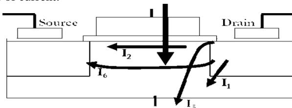
Fig.6: Leakage Power Component
