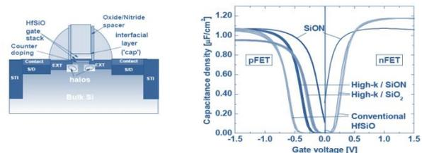
Fig.12: Optimized high-k dielectric stack reduces pFET  $V_t$  shift by 200~300 mV and selective use of ultra-thin interface/surface modification layers and Increased Nitrogen concentration decreases gate leakage current
