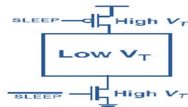
Fig.21: Circuit Design with Sleep Transistors
