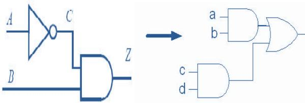
Fig.18: Glitch Free AND Gate as shown in figure above buffers are generally used to delay path A to overcome glitches
