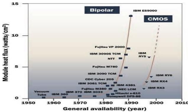
Fig.5: Power dissipation trends, comparison of Bipolar and CMOS technologies.
