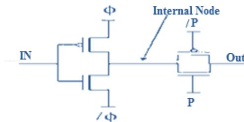
Fig.16: Charge Recovery Logic
