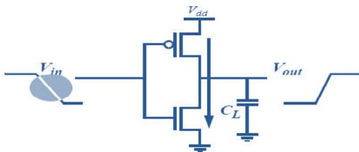
Fig.23: Short Circuit Power in CMOS Circuits
